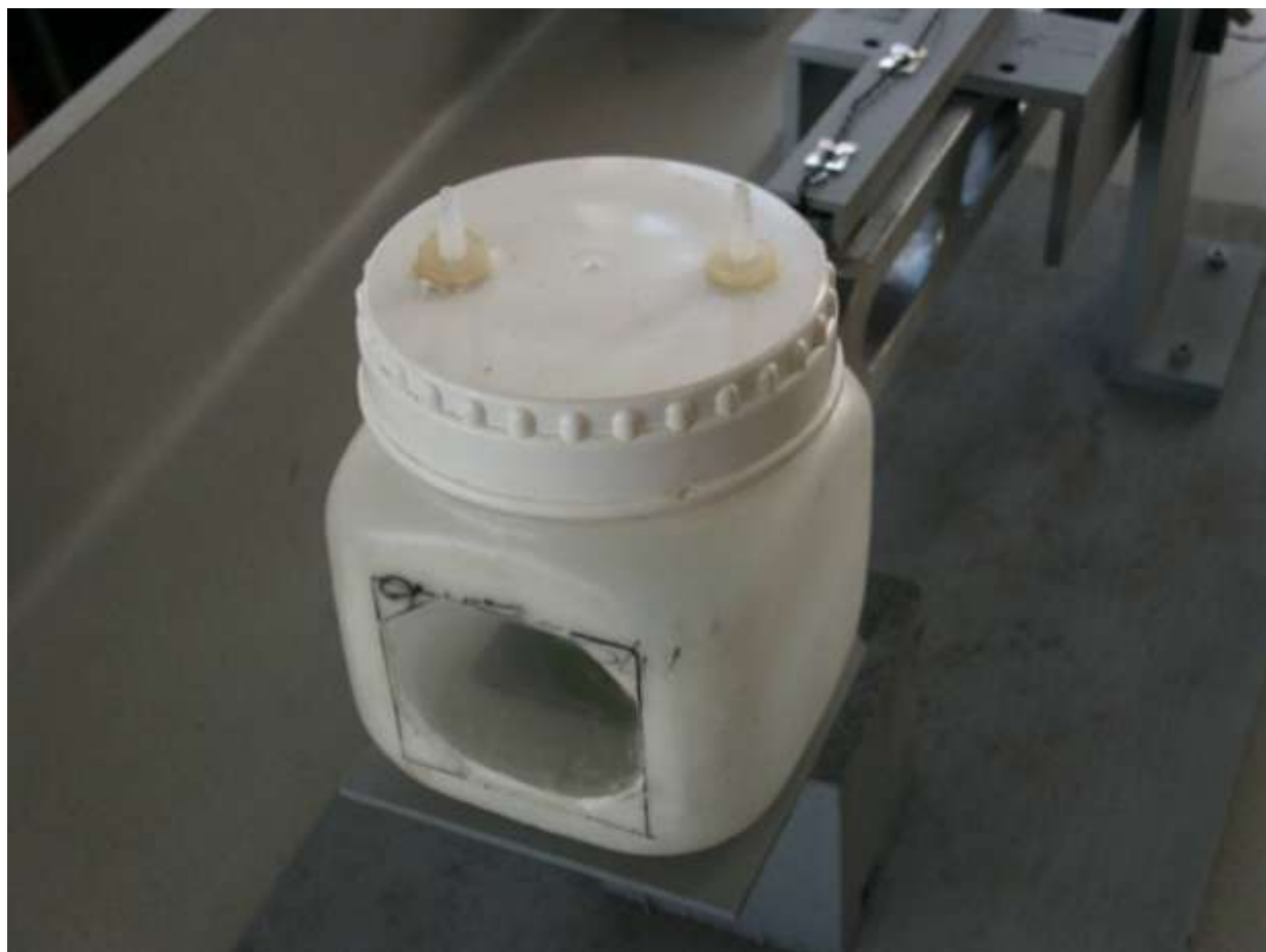
Fig. 4: Plastic container, leaf and invertebrate inside. Air volume removed and CO 2 introduced through the valves in the lid.
