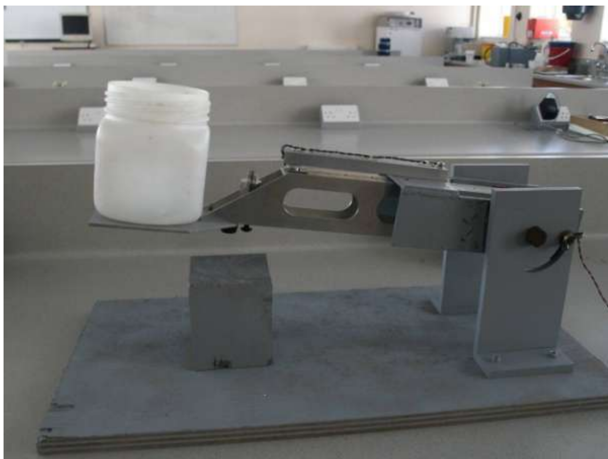
Figure 1: Drop apparatus used to measure the force necessary to dislodge an invertebrate from a leaf
